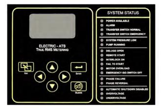
Description-Firetrol® FTA1350 Wye-Delta, Closed Transition Starting Fire Pump Controllers are used with delta-wound squirrel cage motors. FTA1350 controllers are of the closed circuit transition type in which the mo-tor circuit remains closed during the transition from start to run. The controller monitors, displays and records fire pump system information.
